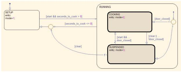
The mode controller starts in the SETUP mode, and transitions to the RUNNING mode when the start button is pressed (if the seconds\_to\_cook parameter is > 0). In the RUNNING mode, the microwave can either be in COOKING or in SUSPENDED mode. If the microwave door is opened when in RUNNING mode or the clear button is pressed, then the microwave is in SUSPENDED mode, where the user can either press the start button to go back to COOKING, or press the clear button again to go back to SETUP.
