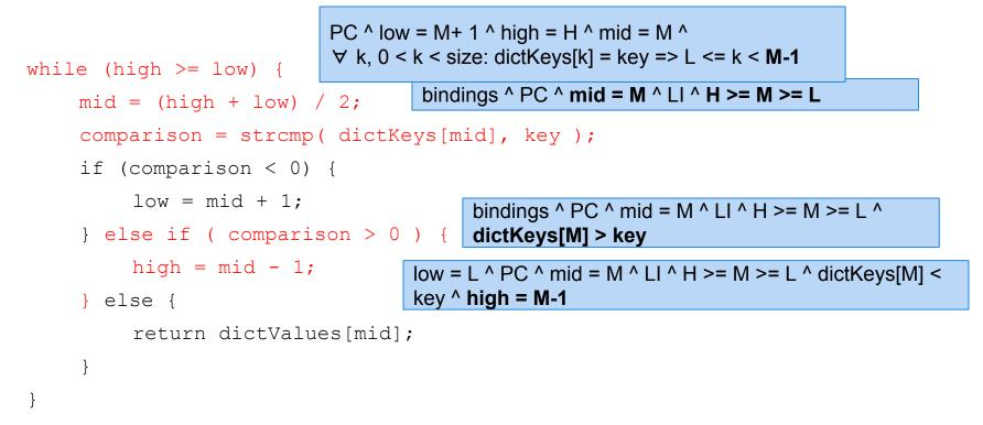
pre-condition (PC):  $\forall$  i, j, 0 <= i < j < size: dictKeys[i] <= dictKeys[j]</th>loop invariant (LI):  $\forall$  k, 0 < k < size: dictKeys[k] = key => L <= k < H</th>bindings: low = L ^ high = H
