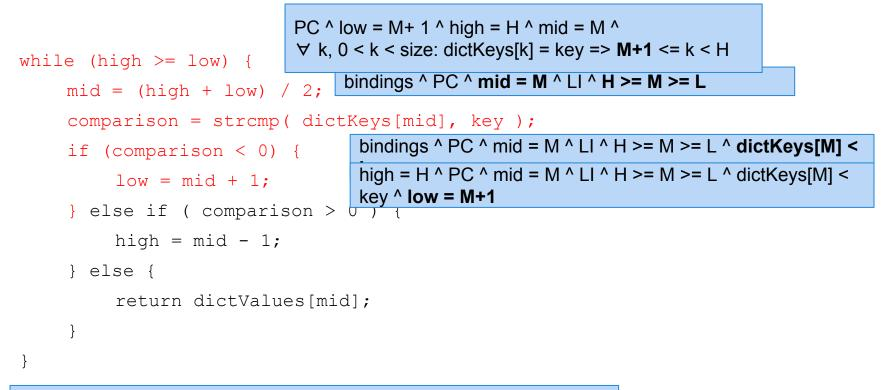
pre-condition (PC):  $\forall$  i, j, 0 <= i < j < size: dictKeys[i] <= dictKeys[j] loop invariant (LI):  $\forall$  k, 0 < k < size: dictKeys[k] = key => L <= k < H bindings: low = L ^ high = H
