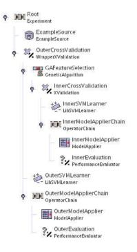
Figure 3. Rapid-I's operator trees. [17]. Internally, this tree is a nested XML expression that is traversed top-down to complete an experiment.
